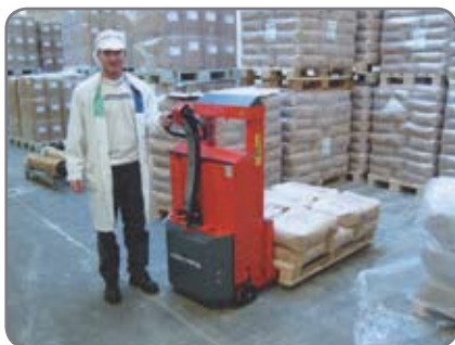
Optimum safety through transparent and impact-resistant safety screen and reduced driving speed in raised position.
