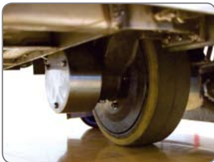
The stainless propulsion motor manages aggressive and wet environments down to -30°.
